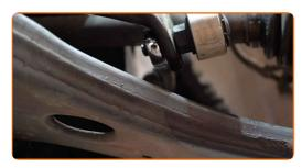
Tighten the fastener connecting the stabilizer link to the shock strut. Use a drive socket #15. Use a torque wrench. Tighten it to 48 nm torque.
