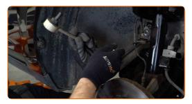
Install a new rod, tighten the fasteners.
