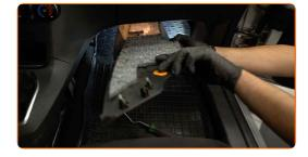
6 Unscrew the fasteners of the cabin filter housing cover. Use Torx T20. Use a ratchet wrench.
