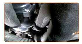
Tighten the EGR valve fasteners. Use a drive socket #8. Use a torque wrench. Tighten it to 9 Nm torque.
