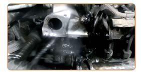
Treat the EGR valve fasteners. Use a sealant.
