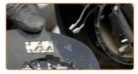
Pry the wing mirror cover clips out of position. Use a plastic trim tool (2 pieces).
