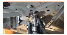
Unscrew the rear fastener connecting the control arm to the subframe. Use a drive socket #13. Use a tap wrench.
