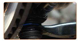
Screw the front arm fastener. Use a drive socket #15. Use a ratchet wrench.
