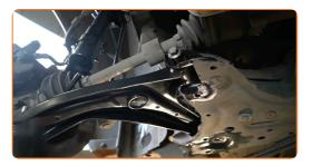
Connect the ball joint to the steering knuckle.
