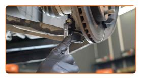
8 Remove the fastening bolt.
