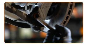
Unscrew the front arm fastener. Use a drive socket #15. Use a tap wrench.
