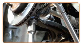
Remove the support from under the arm.
