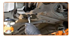
Tighten the rear fastener connecting the arm to the body subframe. Use a drive socket #15. Use a torque wrench. Tighten it to 65 Nm torque.+180°
