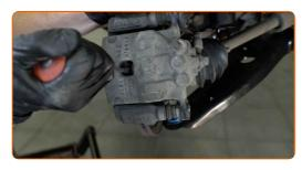
10 Remove the brake caliper.
