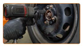
Lower the car and working in a cross order, tighten the wheel bolts. Use wheel impact socket #19. Use a torque wrench. Tighten it to 110 Nm torque.
