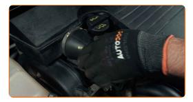
Fasten the clamp on the air intake hose. Use clic-R collar pliers.
