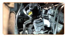
Remove the EGR valve hose clamp. Use clic-R collar pliers.
