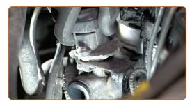
Clean the EGR valve mounting seat. Use all-purpose cleaning spray.
