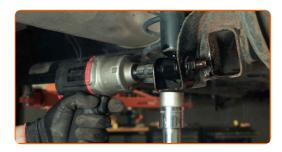
9 Remove the fastening bolt.
