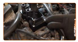
Treat the ignition coil connector with electronic spray.
