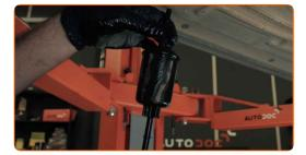
Connect the fuel supply lines to the fuel filter.
