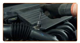
Attach the crankcase ventilation hose to the engine cover at the left.
