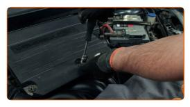
Detach the crankcase ventilation hose from the engine cover at the left.
