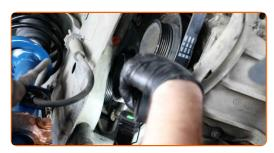
Turn the crankshaft pulley. Use a crowbar. Use a drive socket #18. Use a tap wrench.
