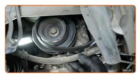
Install the V-ribbed belt. Use a crowbar. Use a drive socket #18. Use a tap wrench.
