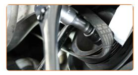
Remove the hydraulic power steering belt.
