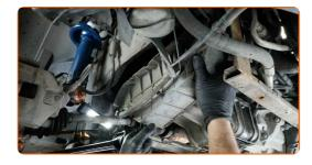
Tighten the fasteners of the oil pan lower cover. Use Torx T27.
