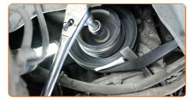
Turn the crankshaft pulley. Use a crowbar. Use a drive socket #18. Use a tap wrench.
