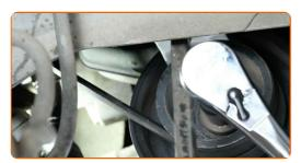
Turn the crankshaft pulley. Use a drive socket #18. Use a tap wrench.
