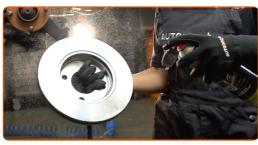
19 Install the brake disc.
