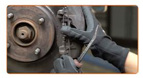
Remove the brake caliper.
