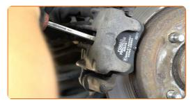
Remove the brake caliper.
