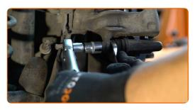
Install the parking brake cable into the brake caliper bracket. Use water pump pliers.
