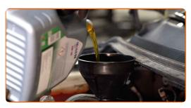
Replacement: engine oil and filter – FORD Fiesta Mk3 Hatchback (GFJ).
