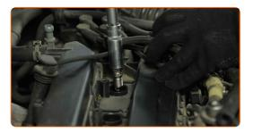
Screw new spark plugs and tighten them. Use the spark plug socket #16. Use a torque wrench. Tighten it to 20 nm torque.
