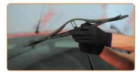
Remove the blade from the wiper arm.
