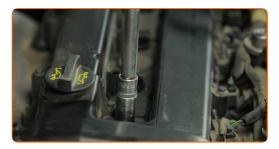
Take out the spark plugs. Use the spark plug socket #16.
