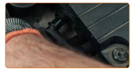
Remove the air intake pipe.
