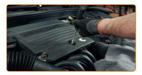
Attach the crankcase ventilation hose to the engine cover at the left.
