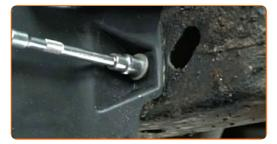
Screw in the fastening bolt of the windscreen washer reservoir's cover. Use a 10 mm socket. Use a ratchet wrench.
