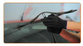
Remove the blade from the wiper arm.
