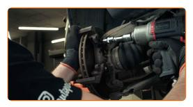
Remove the caliper bracket.
