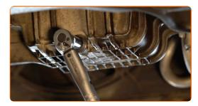
Reinstall the oil pan lower cover. Tighten the fasteners of the oil pan lower cover. Use a drive socket #10. Use a ratchet wrench.
