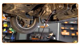
Replacement: engine oil and filter – FORD Escort Mk5 Hatchback (AAL, ABL). Tip:
