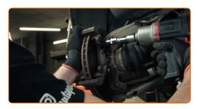
Remove the caliper bracket.
