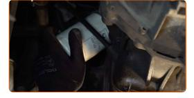
Prepare a container for the old oil filter. Put the old oil filter in the container.
