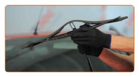
Remove the blade from the wiper arm.
