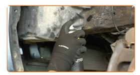
Unscrew the fastening bolt of the windscreen washer reservoir's cover. Use a 10 mm socket. Use a ratchet wrench.
