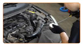
Replacement: engine oil and filter – FORD Escort Mk3 Hatchback (GAA). Tip from AUTODOC:
