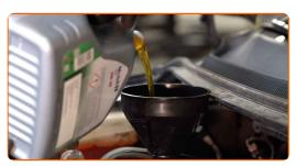
Replacement: engine oil and filter – FORD Escort Mk3 Hatchback (GAA).
