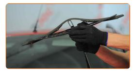
Remove the blade from the wiper arm.
