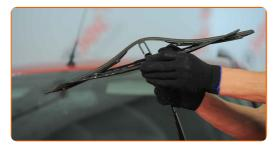
Remove the blade from the wiper arm.
