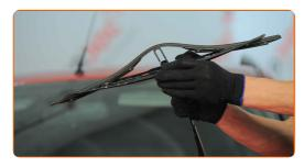
Remove the blade from the wiper arm.
