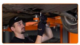
Remove the oil pan cover. Use a drive socket #10. Use a flat screwdriver. Use a ratchet wrench. 6
