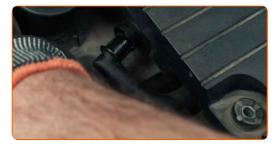
Remove the air intake pipe.
