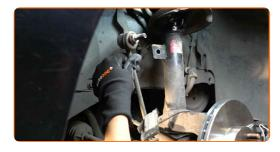
Clean the mounting seats of the stabiliser link. Use a wire brush. Use WD-40 spray.
