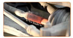
Install a new rod, tighten the fasteners. Use a combination spanner #15. Use a drive socket #15. Use a ratchet wrench.
