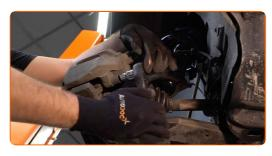
Remove the brake caliper.
