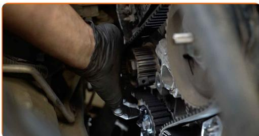
Replacement: water pump & timing belt kit – FORD C-Max II (DXA/CB7, DXA/CEU). Tip from AUTODOC:
