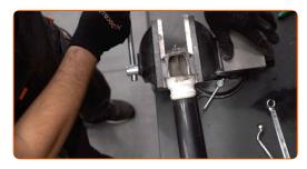
Clean the shock absorber rod fastener. Use a wire brush. Use WD-40 spray. 13
