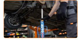
Clean the fasteners of the shock absorber upper mount. Use a wire brush. Use WD-40 spray.
