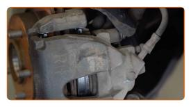
Install the brake caliper retaining spring.
