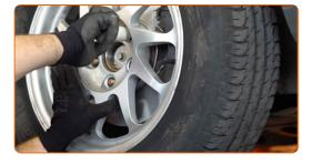
Lower the car and working in a cross order, tighten the wheel bolts. Use a torque wrench. Tighten it to 110 nm 23 torque.
