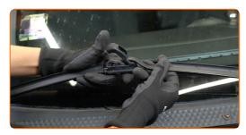
Remove the blade from the wiper arm.
