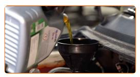
Replacement: engine oil and filter – FORD C-Max (DM2). Professionals recommend:
