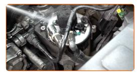
Disconnect the fuel supply lines from the fuel filter. Use a flat screwdriver.
