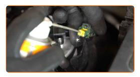
Attach the fuel pressure sensor connector.
