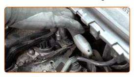
Remove the fuel filter fastening bracket.
