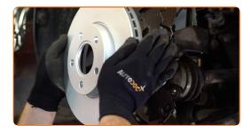
Remove anti-corrosion grease from the new brake disk. Use a brake cleaner.
