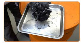
Unscrew the fasteners of the fuel filter housing cover. Use Torx T15. Use a ratchet wrench.
