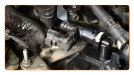
Attach the fuel pressure sensor connector.
