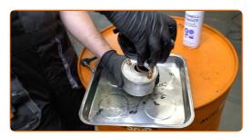
Clean the fuel filter housing and the cover. Use all-purpose cleaning spray.
