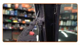
Release the circlip connecting the gas strut to the car body. Use a flat screwdriver.
