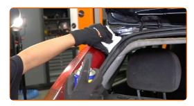
14 Install the new boot lid gas strut.
