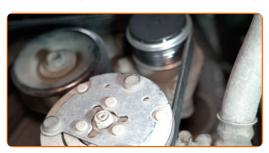
Return the tensioner pulley to its initial position. Use a combination spanner #15.
