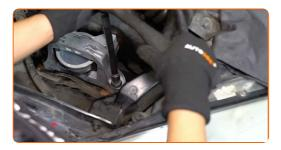
Screw in the upper fastener of the engine mount. Use a drive socket #16. Use a ratchet wrench.
