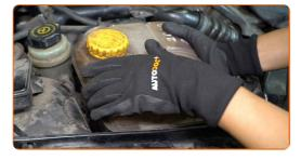
Attach the coolant reservoir using its retainers.
