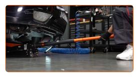
Remove the fender protection cover.
