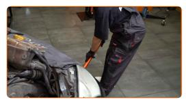
Screw in the fasteners that connect the engine mount to the car body. Use a drive socket #16. Use a ratchet wrench.
