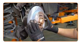
35 Screw in the brake disc fastener. Use a crowbar.
