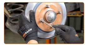
14 Remove the brake disc.
