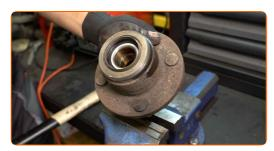
Remove the wheel hub bearing retaining ring. Use circlip pliers.
