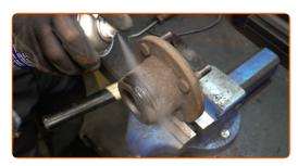
Remove the inner wheel bearing oil seal. Use a crowbar. Use a hammer.
