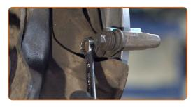
Remove the caliper bracket.
