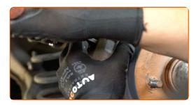
Remove the brake caliper.
