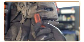
Unscrew the brake caliper fastening. Use a combination spanner #15. Use a drive socket #13. Use a ratchet wrench.
