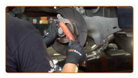
34 Install the brake disc.
