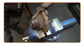
Loosen the vice and remove the hub.
