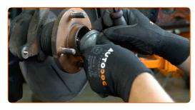
Unscrew the hub nut. Use a drive socket #30. Use a tap wrench.
