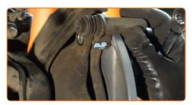
Unscrew the brake disc fastening. Use a flat screwdriver.
