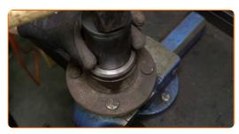
Clean the hub bearing mounting seat. Use a wire brush. Use all-purpose cleaning spray. Use WD-40 spray.
