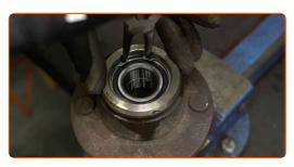
Press in the inner wheel bearing oil seal. Use a bush and bearing driver set. Use a hammer.
