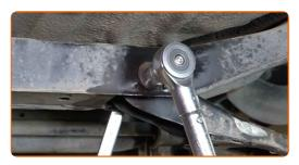
Tighten the fastener connecting the suspension arm to the rear knuckle. Use a drive socket #15. Use a torque wrench. Tighten it to 85 Nm torque.
