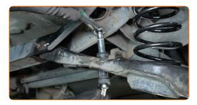
Treat all joints of the arm. Treat all joints of the stabiliser link. Use copper grease.
