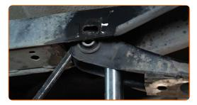
Install the fastening bolt. Use a combination spanner #19.
