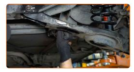
Tighten the fastener connecting the stabilizer link to the stabilizer bar. Use a combination spanner #13. Use a drive socket #13. Use a torque wrench. Tighten it to 15 Nm torque.
