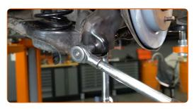
Remove the support from under the arm.
