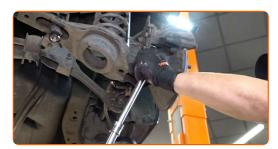
Unscrew the fastener connecting the stabilizer link to the stabilizer bar. Use a combination spanner #13. Use a drive socket #13. Use a ratchet wrench.
