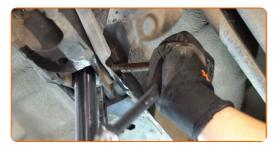
Remove the support from under the arm. Use a crowbar.
